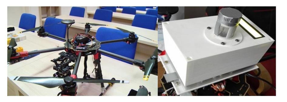
4 temperature sensors; Sensor of relative humidity; barometer; accelerometer (3D), gyroscope (3D), magnetometer (3D); 2 optical particulate sensors (PM1, PM2.5, PM10); 5 electrochemical sensors (NO, NO2, O3, SO2, CO)
